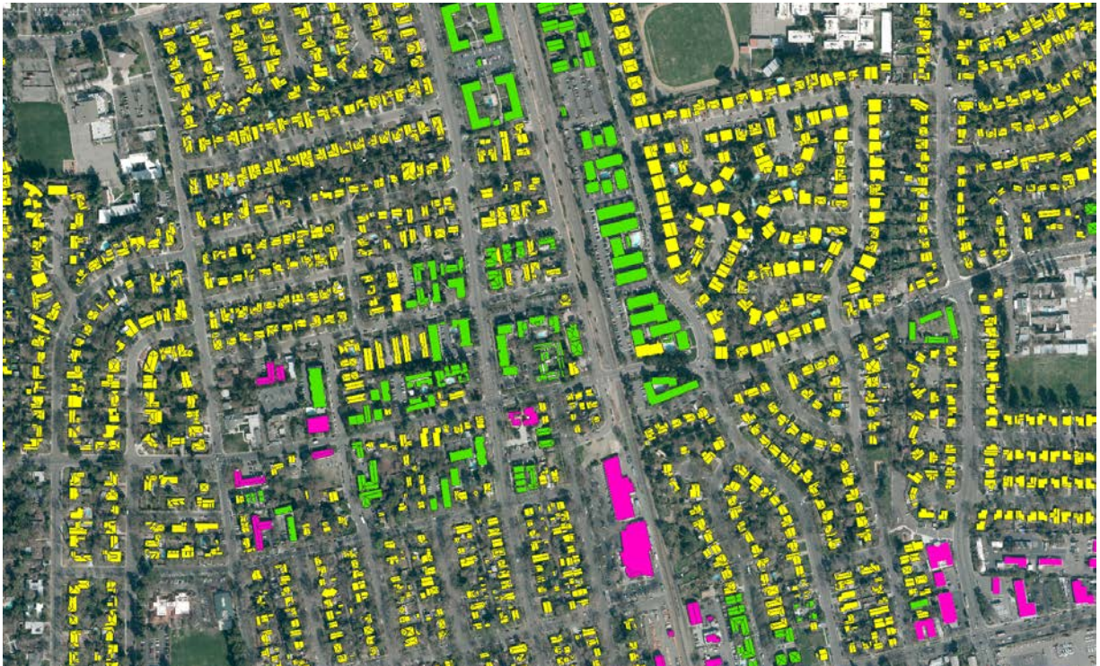
Figure 17: Davis PV Rooftop Usable Area Digital Photo – Closer View
